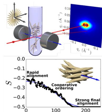
Figure 1. Experimental SAXS setup and evolution of order parameter over time showing cooperative ordering of a CNC chiral nematic suspension.
