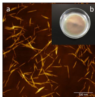
Figure 1. AFM image of CNCs (a) and their chiral phase (b).
